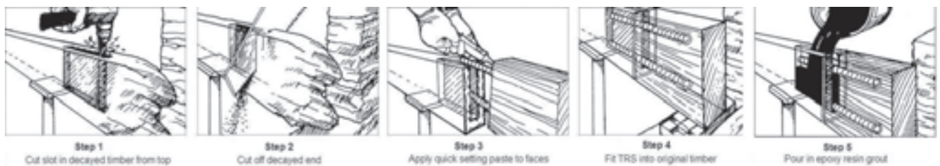
Figure 7. TRS repair stages
